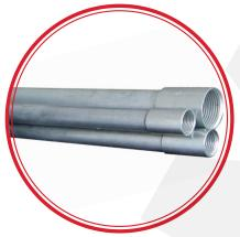
IMC (intermediate metal conduit) is a robust steel electrical conduit that is designed for outdoor use and strong connections. It was created to safeguard insulated electrical wires and cables. It performs the same functions as rigid metal conduit (RMC), but weights roughly a third less. It can be removed the requirement for a heavier-walled conduit by using IMC in any places where it is permitted.
